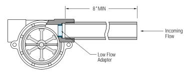
Except for straight-thread versions, RotorFlow sensors connect to piping via NPT mating thread forms. The use of an appropriate thread sealant is necessary to assure a leak-tight connection. Permatex "No More Leaks®" or 2 wraps of Teflon® tape are the only sealants recommended for GEMS flow sensors. Straight-thread versions require an O-ring for sealing.
